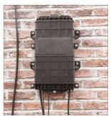
PBO G is an Optical Terminal Point with an integrated 1 x 8 SC/APC splitter and SC/APC adapters for the connection of pre-terminated optical drop cables. Developed as a multiapplication product solution, this optical distribution box made of polypropylene (PP) enables the transition, the termination of the fibre extraction out of a distribution cable with a maximum Ø 9mm.
